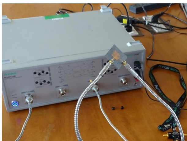
Fig.7 The fabricated antenna with the measurement setup
