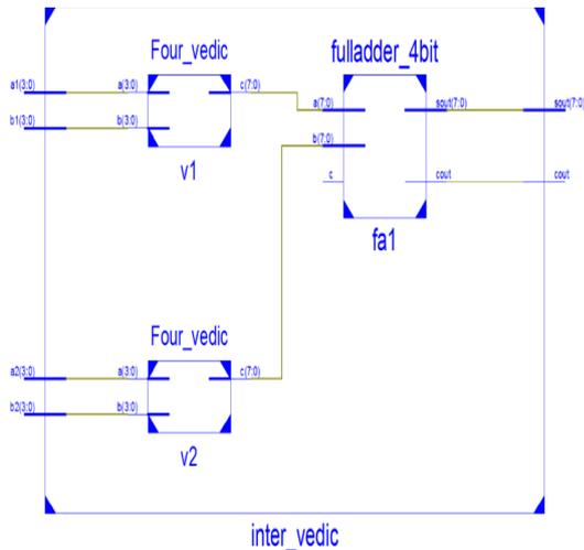
Fig 5 Fir Filter basic unit using Vedic multiplier and full adder
