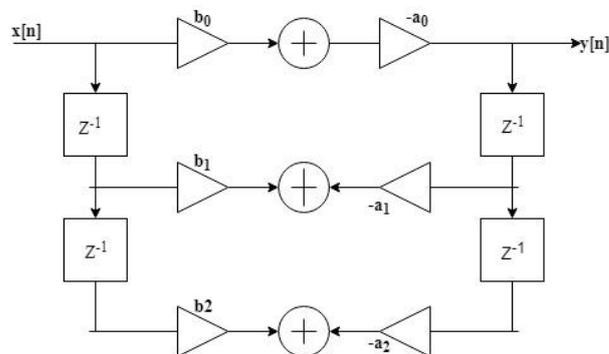
Fig 2 Infinite Impulse Response Filter
