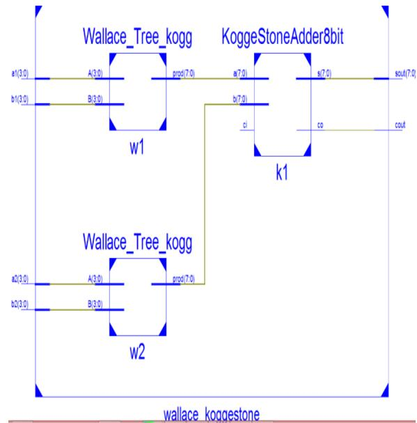
Fig 7 RTL schematic for a Wallace tree and Kogge stone adder
