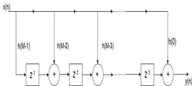
Fig 1 Finite Impulse Response Filter
