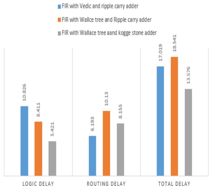
Fig 11 Delays for various Fir Filters
