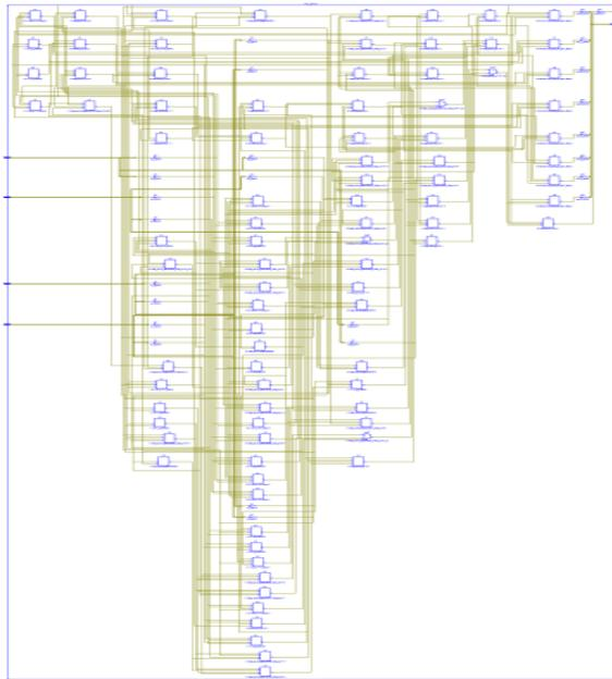
Fig 6 LUT structure of FIR filter using Vedic multiplier and full adder
