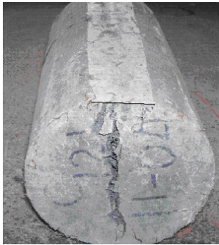
Fig. 2 Fibre based cylinder after split tension test
