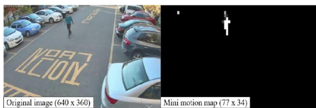
Figure 5: Mini motion map for minimizing the undesirable calculation in HOG dependent person detection. (a) Original image with a size of 640 \times 360 , and (b) mini motion map with a size of 77 \times 34 , which was estimated from GMM-base movement detection
