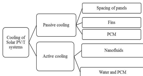
**Figure 2. Different cooling methods of Solar PV/T**
