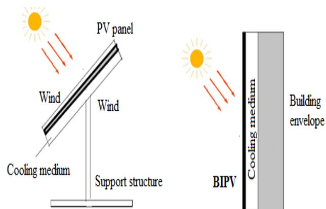
**Figure 1. Cooling of PV panel by cooling medium**
