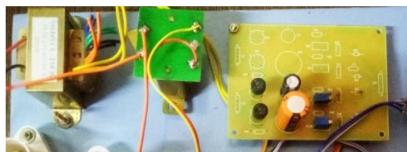
Fig. 2. Picture of PT,CT sensors
