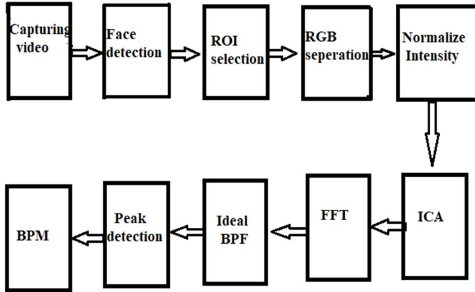
Fig :1 Work flow of proposed method for the measurement of BPM
