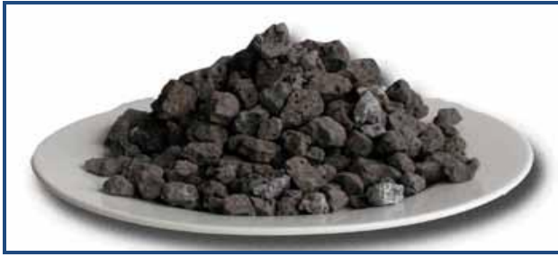
Fig. 2 sorted steel slag to utilize in concrete as coarse aggregates
