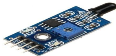
Fig 3: Picture of Fire sensor
