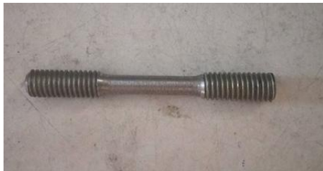
Fig1: The Specimens after machined by varying cutting parameters.
