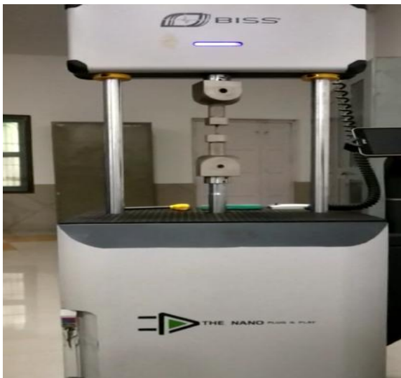
Fig 4: The specimen is undergoing the fatigue test
