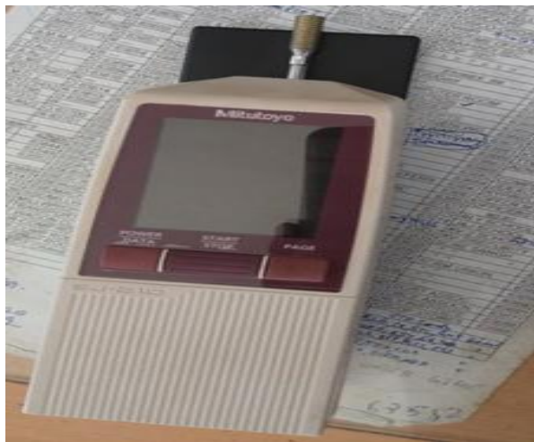
Fig 3: Surface Roughness Calibration of machined specimens
