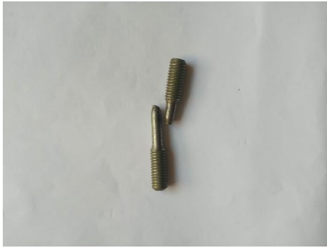
Fig 5: The specimen failure after the fatigue analysis
