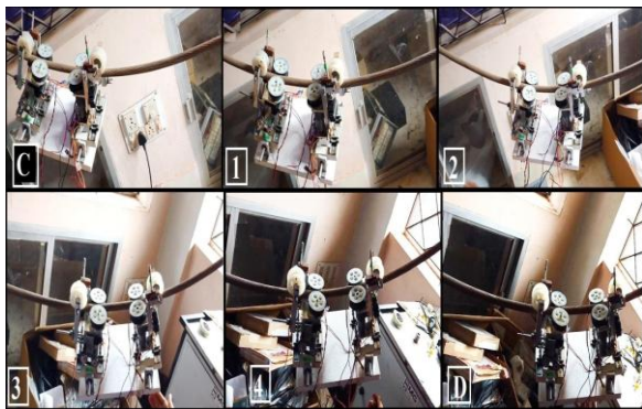
Fig.12. Testing of robot on Sagging line (C-1-2-3-4-D)
