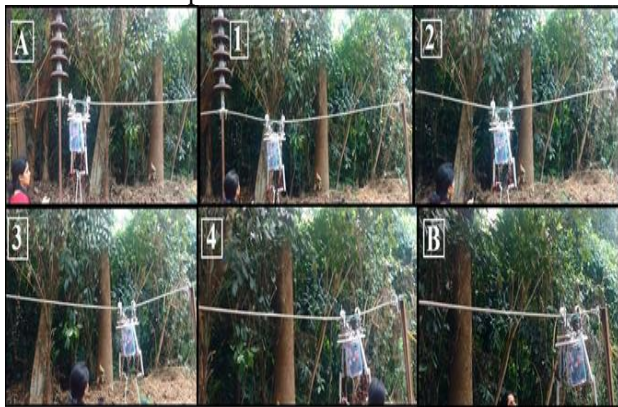
Fig.11. Snapshots taken while testing of robot on the straight transmission line (A-1-2-3-4-B)
