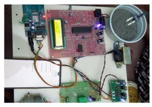
This output shows that GSM is connected to the microcontroller when the soil sensor senses the moisture level it sends a message to the mobile phone.
