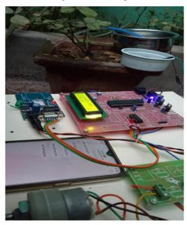
This output shows the result as when the soil is dry the motor on and the water is pumps out to the soil. The message will be sent to the phone.
