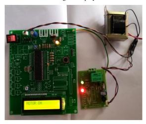
This output shows that, when the power is turn ON, motor starts to run the, in the initial condition relay act as a motor, and the LCD display the message as motor on.
