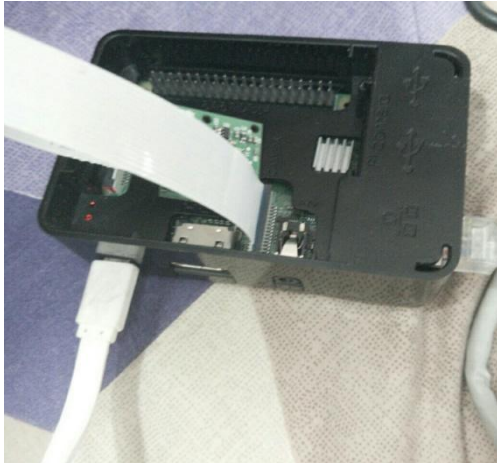
Fig. 1. The Raspberry pi camera setup used for acquisition of vein image.
