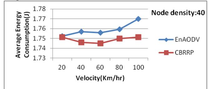
Fig.1. Impact of different velocities on Energy Consumption.
