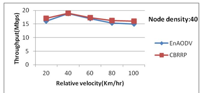
Fig.2. Impact of different velocities on Throughput.
