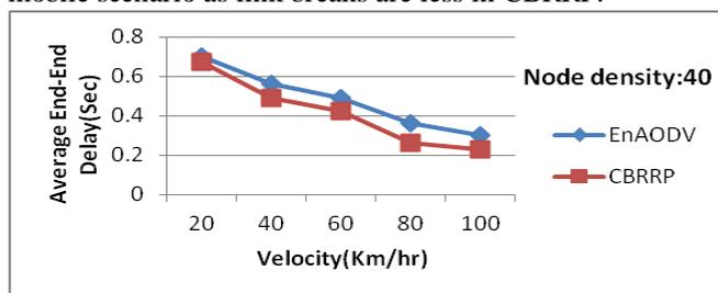
Fig.3. Impact of different velocities on packet delay.
