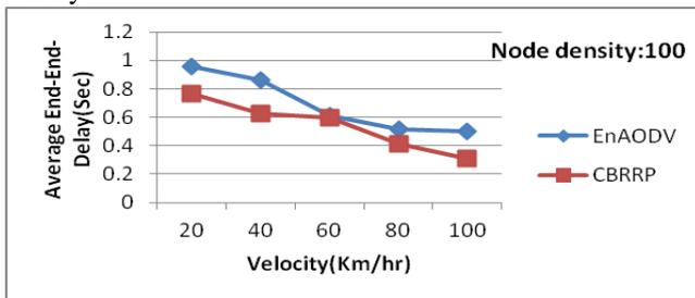
Fig.7. Impact of different velocities on packet delay.
