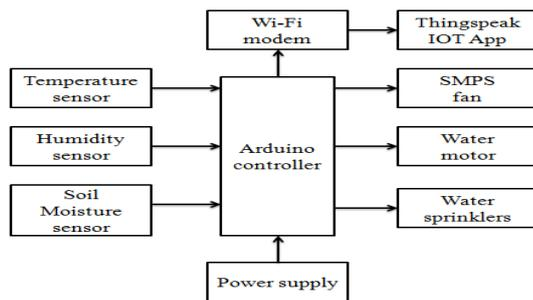
Fig.1 Block Diagram of Home Automation using IoT
