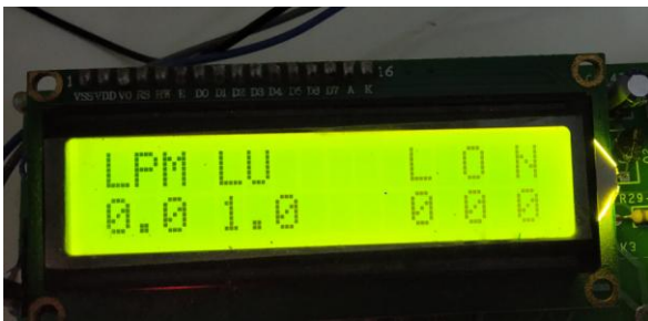
Fig. 4. LCD with LPM, LU and Alert values (in binary)
