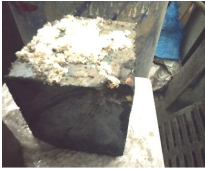
Fig. 2: Sulphate resistance specimen at 90 days
