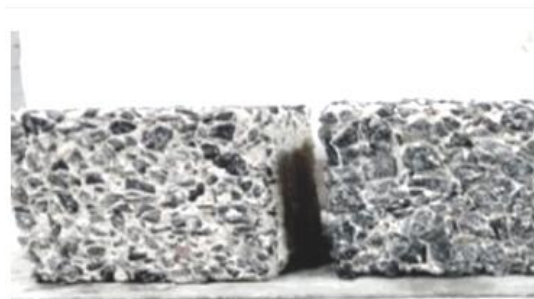
Fig. 1: 56 day Specimen of Acid Attack
