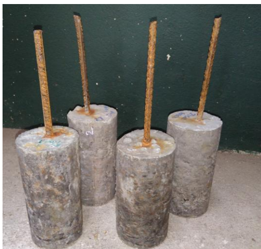
Fig. 3: Salt Spray test Specimen after 168 hours test
