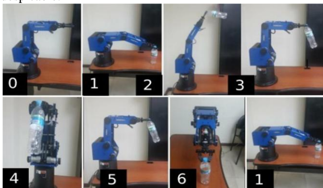
Fig. 9. Programming sequence executed from the client.
