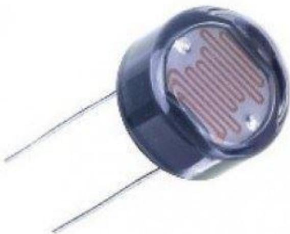
Fig. 4: LDR(Light Dependent Resistor)
