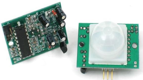
Fig. 3: Passive IR Motion Sensor
