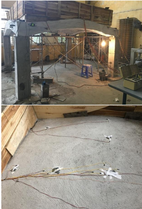
c) The measuring device and strain gages on shell surface
