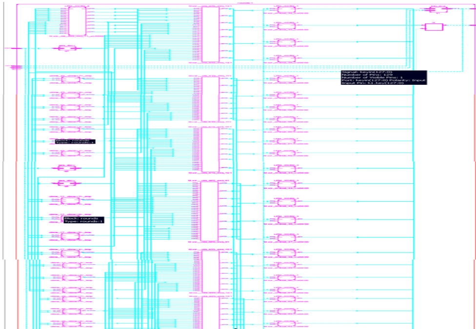
Fig. 4 RTL view of AES FPGA
