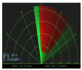
When the object is detected, the screen will display the presence of the object and the angle and distance of the object will also be displayed.
