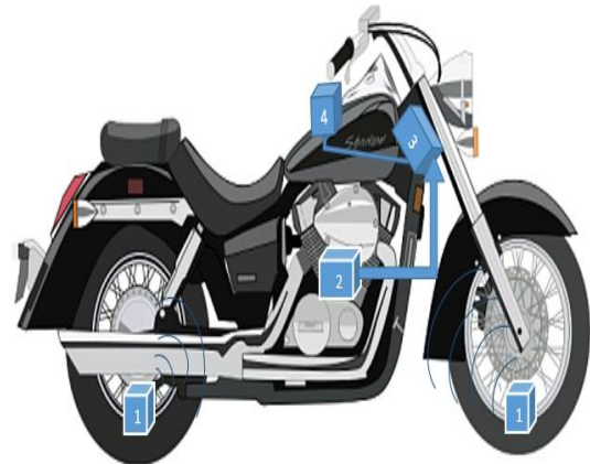
Fig. 5 WTPMS fixed at bike tyre
