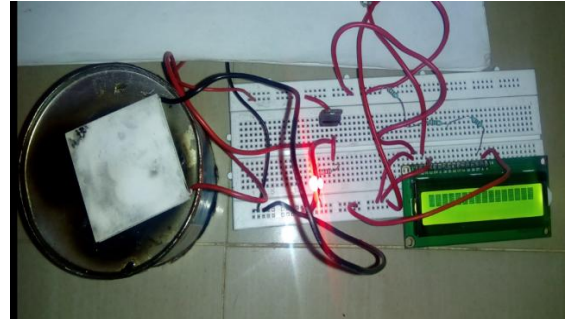
Fig. 7 Generation of electricity from TEC1-12706 Peltier module
