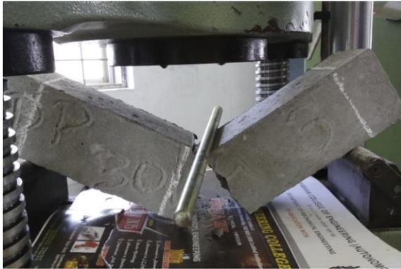
Fig. 8 Flexural test for prism
