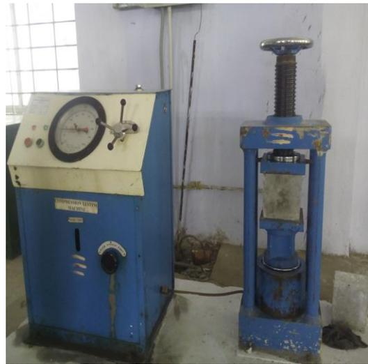
**Fig. 7 Compression testing machine**
