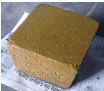
Fig. 9 Acid attack on cube
