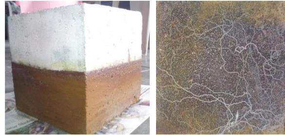
Fig. 10 Sulphate attack on cube
