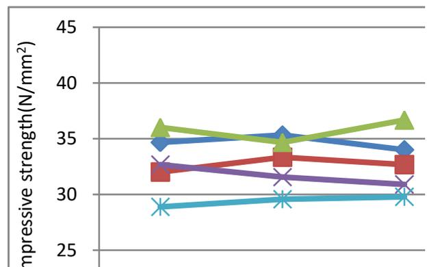
Fig. 12 Comparison chart for 28days cube test results
