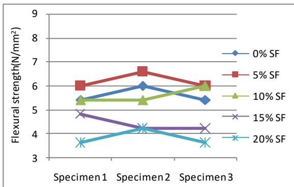
Fig. 14 Comparison chart for 28days prism test results
