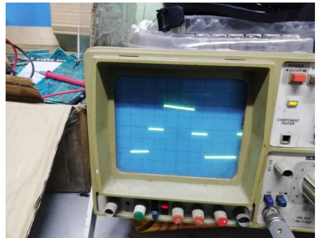
Fig. 9 AC output voltage waveform
