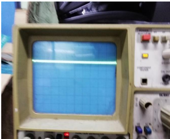
Fig. 17 PV output Voltage waveform
