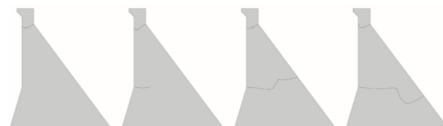
Fig. 6. The destruction of the Guandi Dam under the effect of Koyna earthquake [3]
