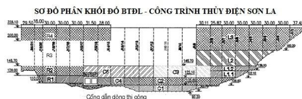
Fig.10 Diagram of dam construction block
