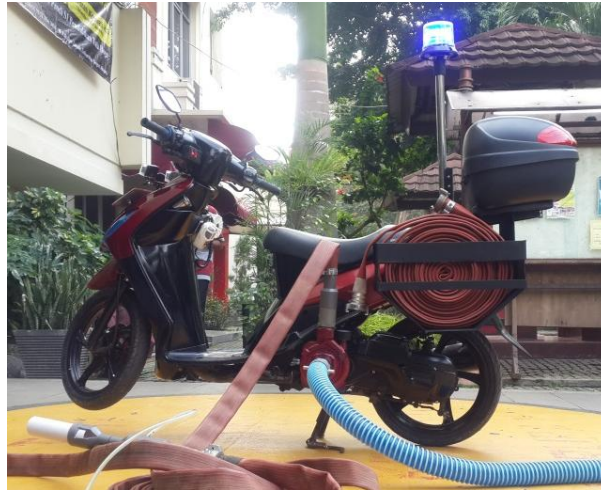
Fig. 7. Installation of firefighter motorcycle
