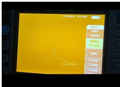
Fig. 14 0.0598 inch of crack
