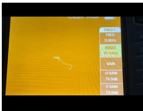
Fig. 15 0.1601 inch of crack
