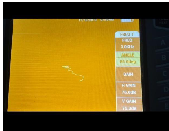
Fig. 15 0.1601 inch of crack
