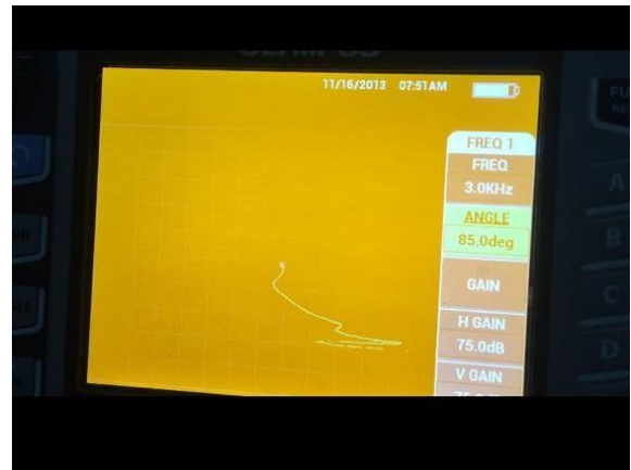
Fig. 14 0.0598 inch of crack
