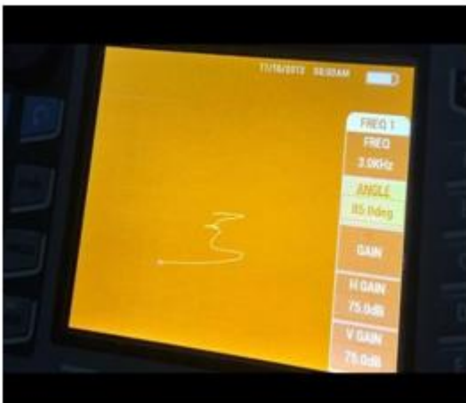
Fig. 12 20% of material loss
