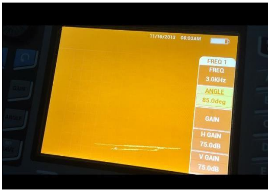
Fig. 11 10% of material loss
