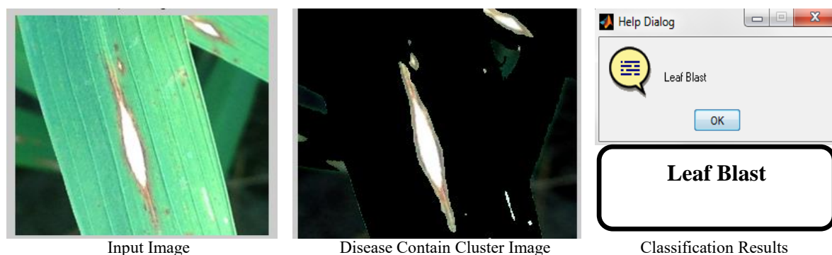
Fig. 10 Input Image, Disease Contain Cluster & Classification Results of Leaf Blast Disease Infected Rice Crop Leaves.
