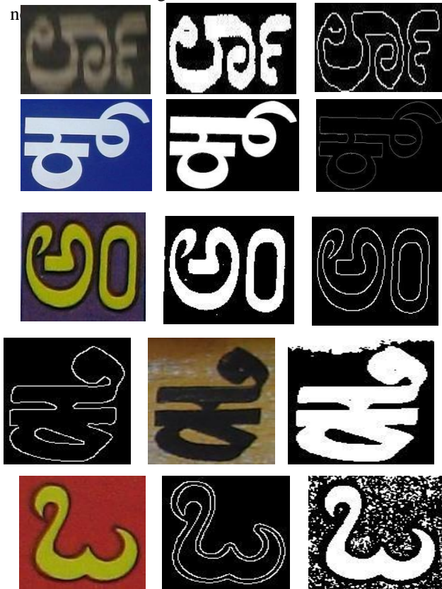
Figure 2: Illustration of preprocessing stages of character Ja. (a) Original Image (b) Binarization (c) Filtered and Morphological Image sampled data sample. (d) Size normalized data sample.
