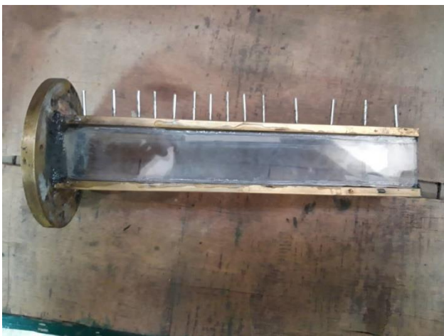
Fig. 5 A view of the Nozzle and the duct assembly
