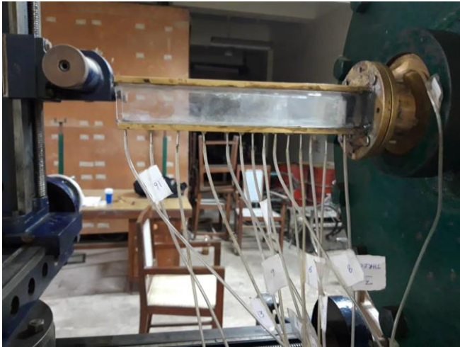
Fig. 4 A view of the Nozzle along with the duct attached with the settling chamber of the open jet facility
