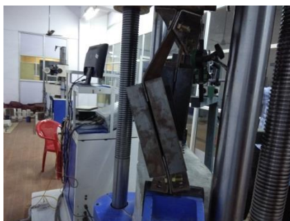
Fig.3 Shear failure of the truss specimen at top corner joint
