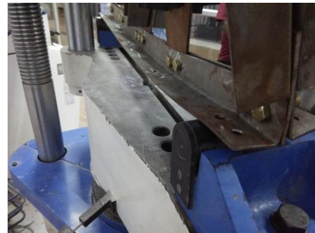
Fig.4 Bending or sagging failure of the truss specimen at bottom mid span
