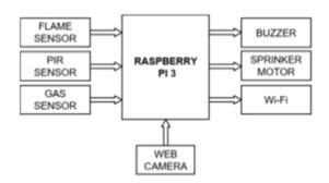
The architecture diagram is almost self explanatory. The sensors and the camera act as input devices that gives input data to the raspberry pi which then processes the information and deduces through the unique algorithm whether there is a fire or not. The buzzer and spikler are close vicinity warning and countermeasure system while the wifi is used to send a message to the security guard and the nearest fire department.
