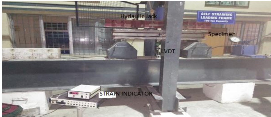
Fig 4 Experimental set-up for the test specimen
