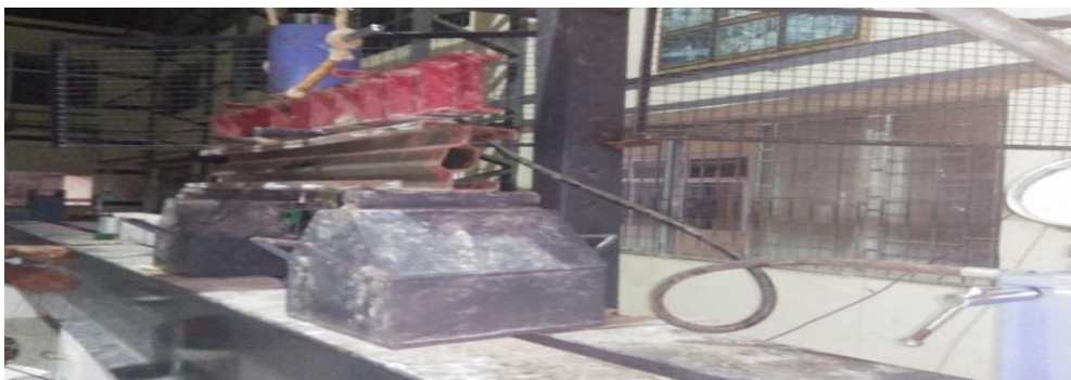
Fig 5 Deflection of Horizontally corrugated beam without spacing
