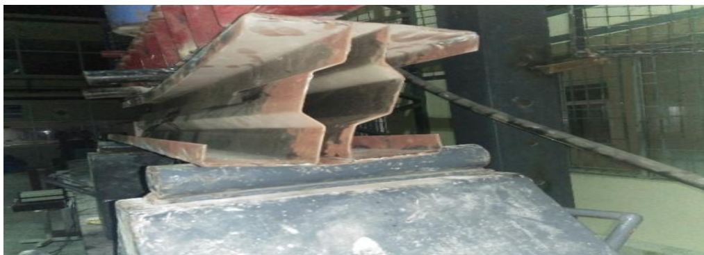
Fig 6 Deflection of Horizontally corrugated beam with a spacing of 25mm
