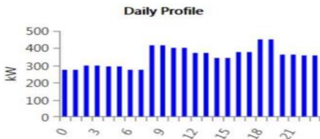
Fig. 3 The daily load profile with Y axis denoting the average power in Kilowatt and X axis denoting the time in hrs.
