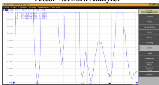
Fig. 9 VSWR curve of the Spiral Antenna from Vector Network Analyzer
