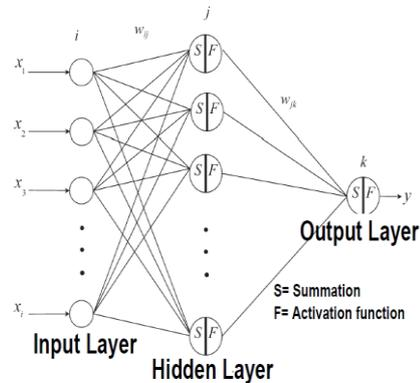
Fig: 2 Representation of Back propagation algorithm
