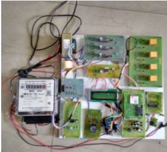
Fig .6 : Hardware Receiver section
