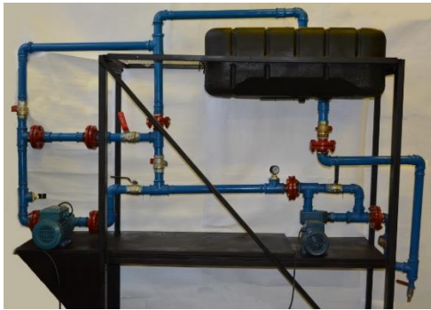
Рис. 2 Model of experimental bench for recycling oil wastes
