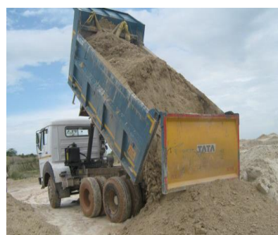
Fig. 1.3&1.4 Truck loaded with phosphogypsum in Phosphoric Acid plant and unloading in phosphogypsum stack area (Dry stacking)
