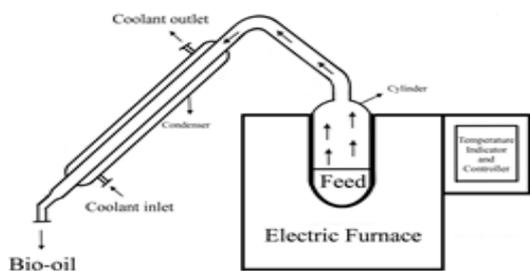
Figure 1. Experimental set-up for recovery of bio-oil
