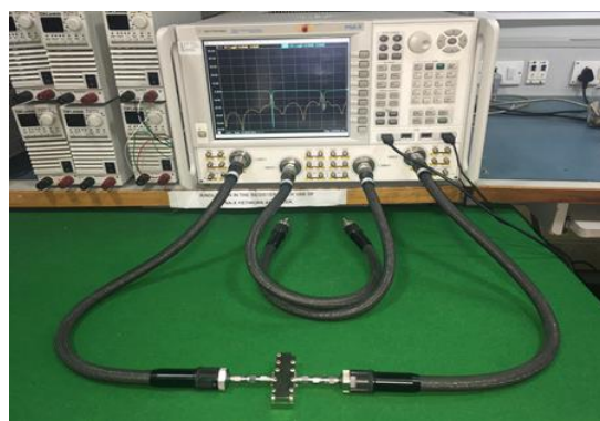
Figure.10 2-Port Configured online Measured return loss and insertion loss of Proposed Dual Notch Filter
