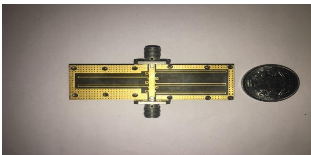
Figure.8 Photograph of the Fabricated Dual Notch unit (Top-View).The Photograph Indicates the Compact Dimensions With One Rupee Coin.
