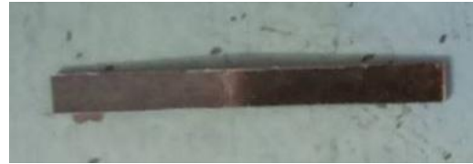
Fig. 2. Sisal Fiber composite sample for three point flexural testing
