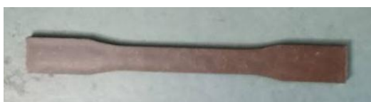
Fig. 1. Sisal Fiber composite sample as per ASTM standard for tensile testing
