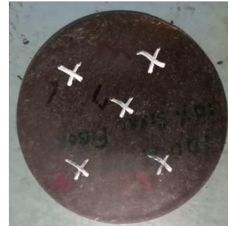
Fig. 3. Sisal Fiber composite samples for hardness testing with five points marked for testing
