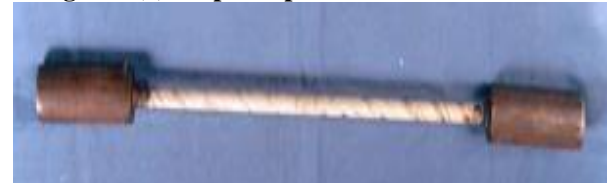
Figure 2(b) Grip Setup of Grooved GFRP
