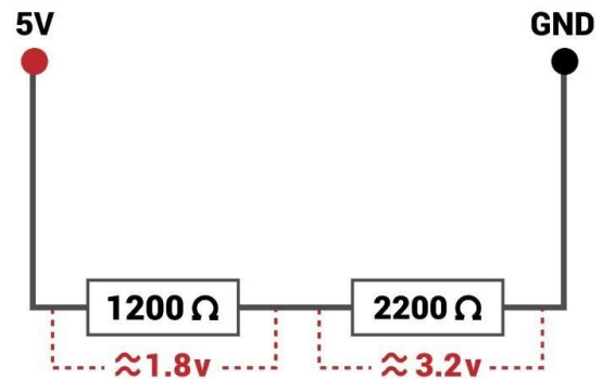
Fig. 4. Potential Divider
