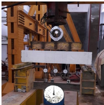
Figure 5 Testing of Beam Under Two Point Loading
