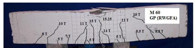
Figure 17 Crack Patterns of M 60 GP (RWGFA) Beam
