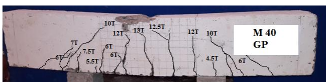
Figure 13 Crack Patterns of M 40 GP Beam
