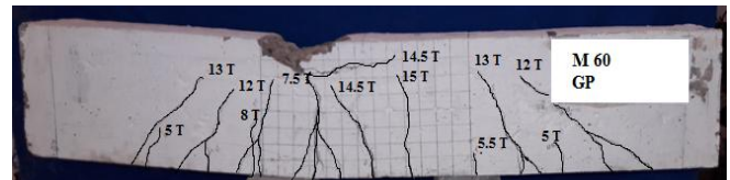
Figure 16 Crack Patterns of M 60 GP Beam
