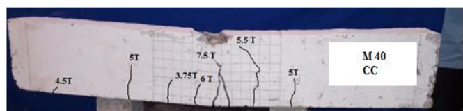
Figure 14 Crack Patterns of M 40 CC Beam
