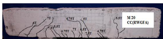
Figure 13 Crack Patterns of M 20 CC (RWGFA) Beam
