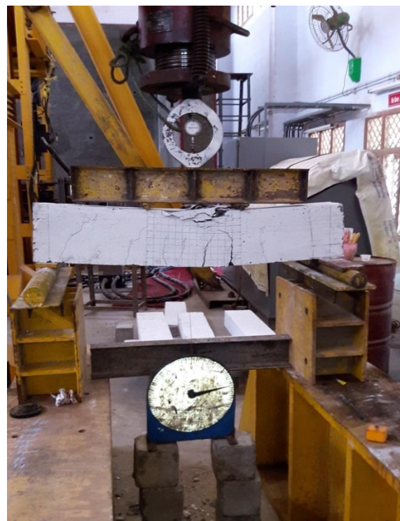
Figure 5 Testing Specimen Under Two Point Loading Table 7 Test Result of Cement Concrete and RWGFA Concrete Beams
