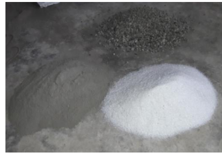
Figure 3 Materials used for RWGFA Geopolymer Concrete
