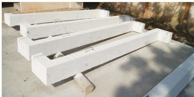
Fig. 2 Cast specimen for torsional test
