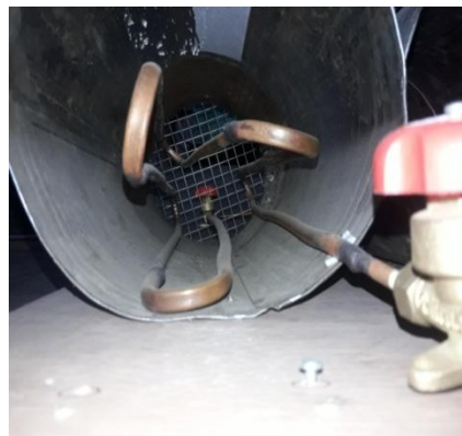
Fig. 4: Condensers tubes are placed in the shell
